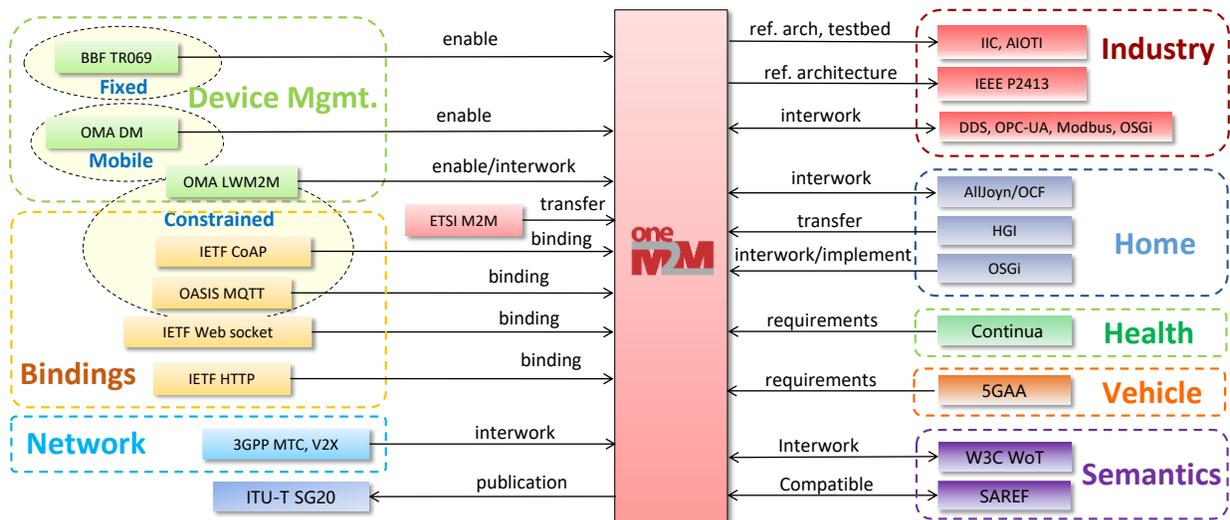
Figure 11 oneM2M role as an interoperability hub across industries and industry-specific protocols (Source: oneM2M)
