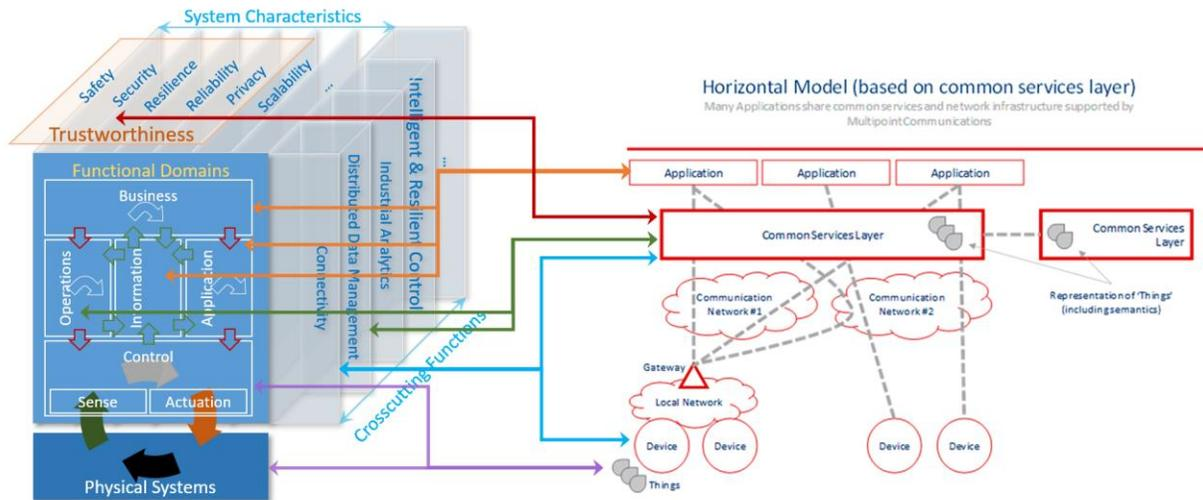
*Figure 7 IIRA functional domain and oneM2M high-level service mapping*
