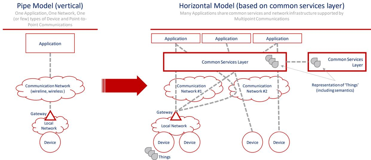
Figure 4 Overview of oneM2M Horizontal Architecture (Source: oneM2M)
