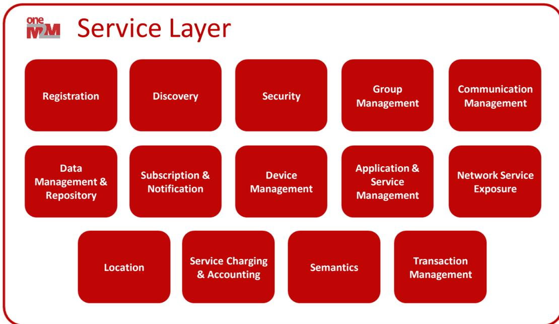
Figure 5 oneM2M Common Service Layer Functions (Source: oneM2M)
