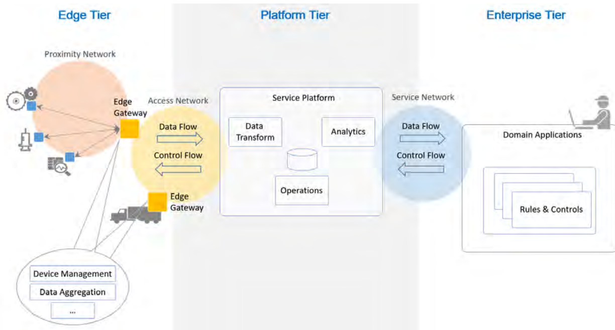
Figure 7-1: Three-Tier IIoT System Architecture
